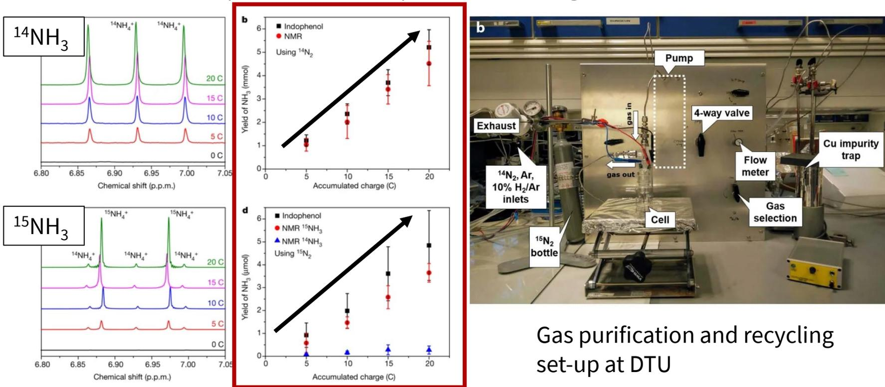
Gas purification and recycling set-up at DTU
