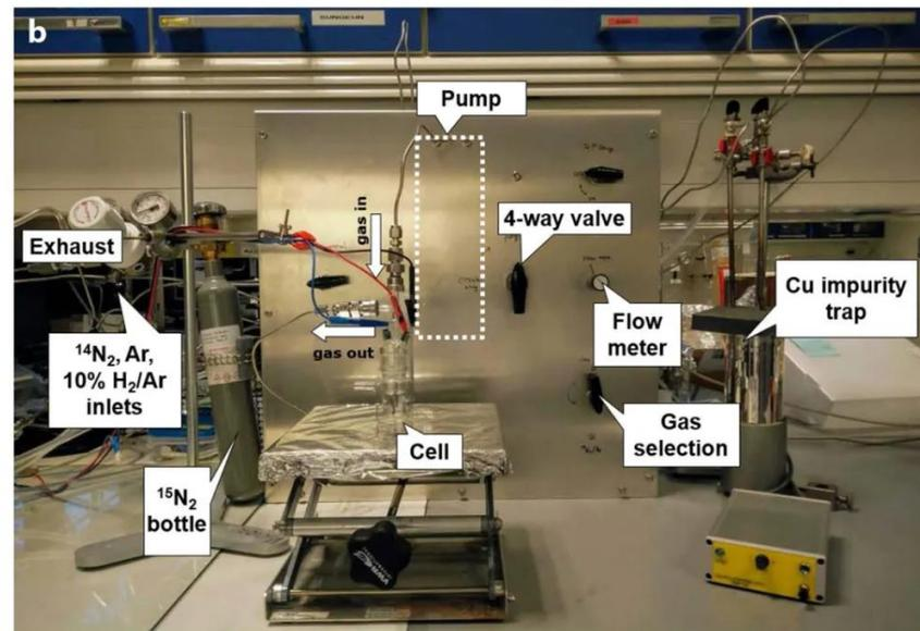
Gas purification and recycling set-up at DTU
