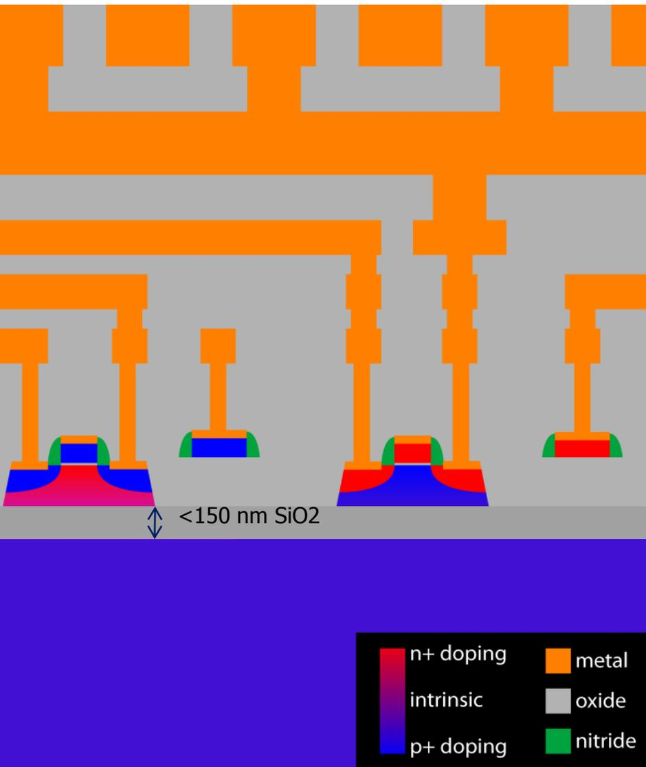
Thin BOX SOI CMOS Electronics
