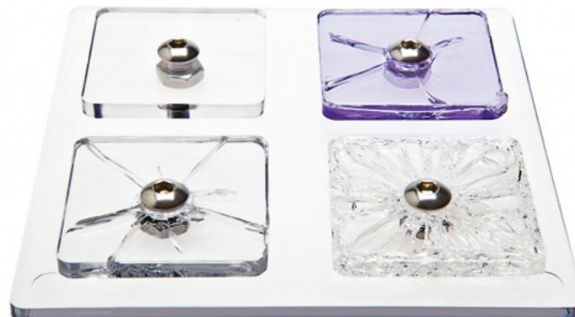
Analysis of Environmental Stress Cracking on Plastic Surface
