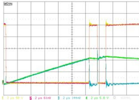
Double pulse test cycle, showing initial current ramp followed by rapid on/off pulse to test DUT switching under full current conditions. Calibration of on-board current measurement circuit (Ch.3 blue) against an Agilent hall-effect current probe (Ch.4 green).
