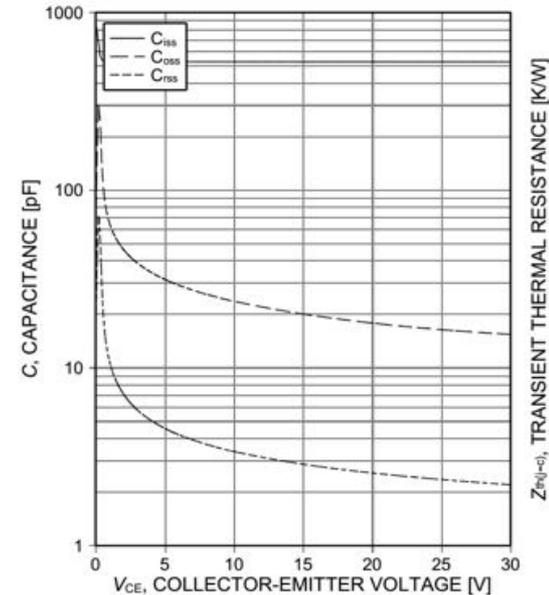
Figure 17. Typical capacitance as a function of collector-emitter voltage ( $V_{GE}=0\text{V}$ ,  $f=1\text{MHz}$ )
