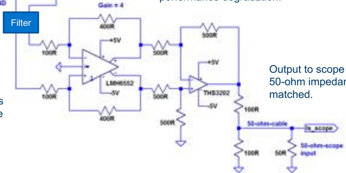
Output to scope is 50-ohm impedance matched.
