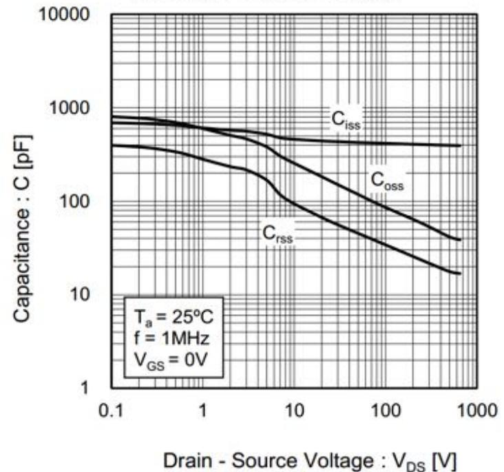
The SiC MOSFET capacitances can contribute to significant ringing.
