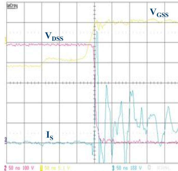
The  $dV/dt$  is around  $50,000\text{V}/\mu\text{s}$ , virtually no overshoot.
