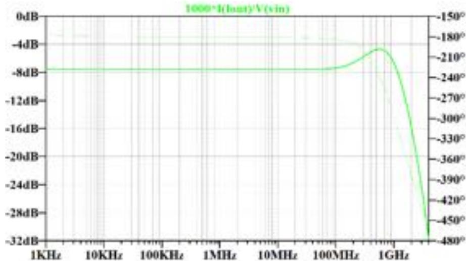
*Gate-drive test with VNA 1MHz-1GHz*
