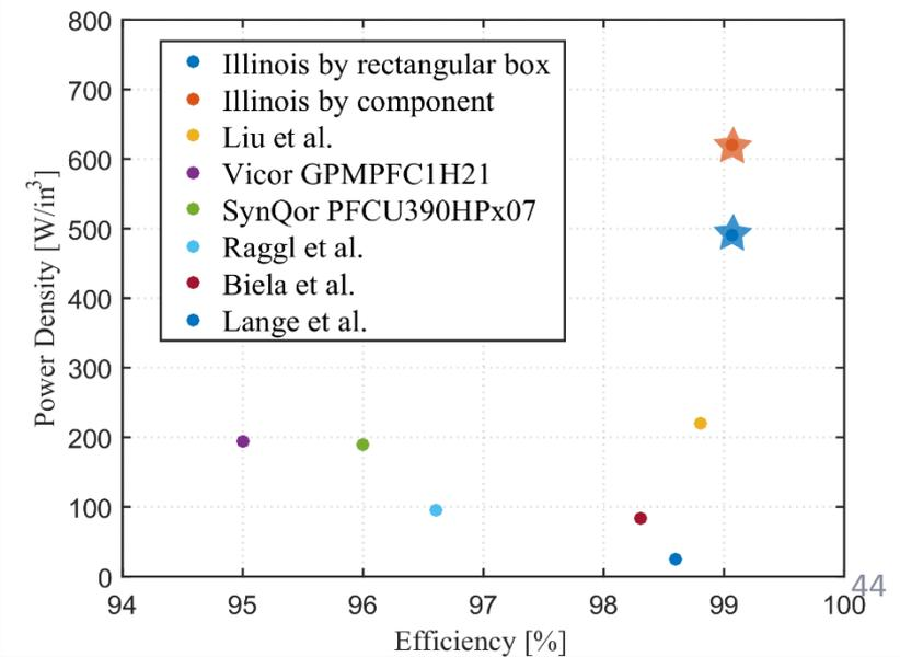
Liu et al., Design of GaN-based mhz totem-pole PFC rectifier, JESTPE 2016
