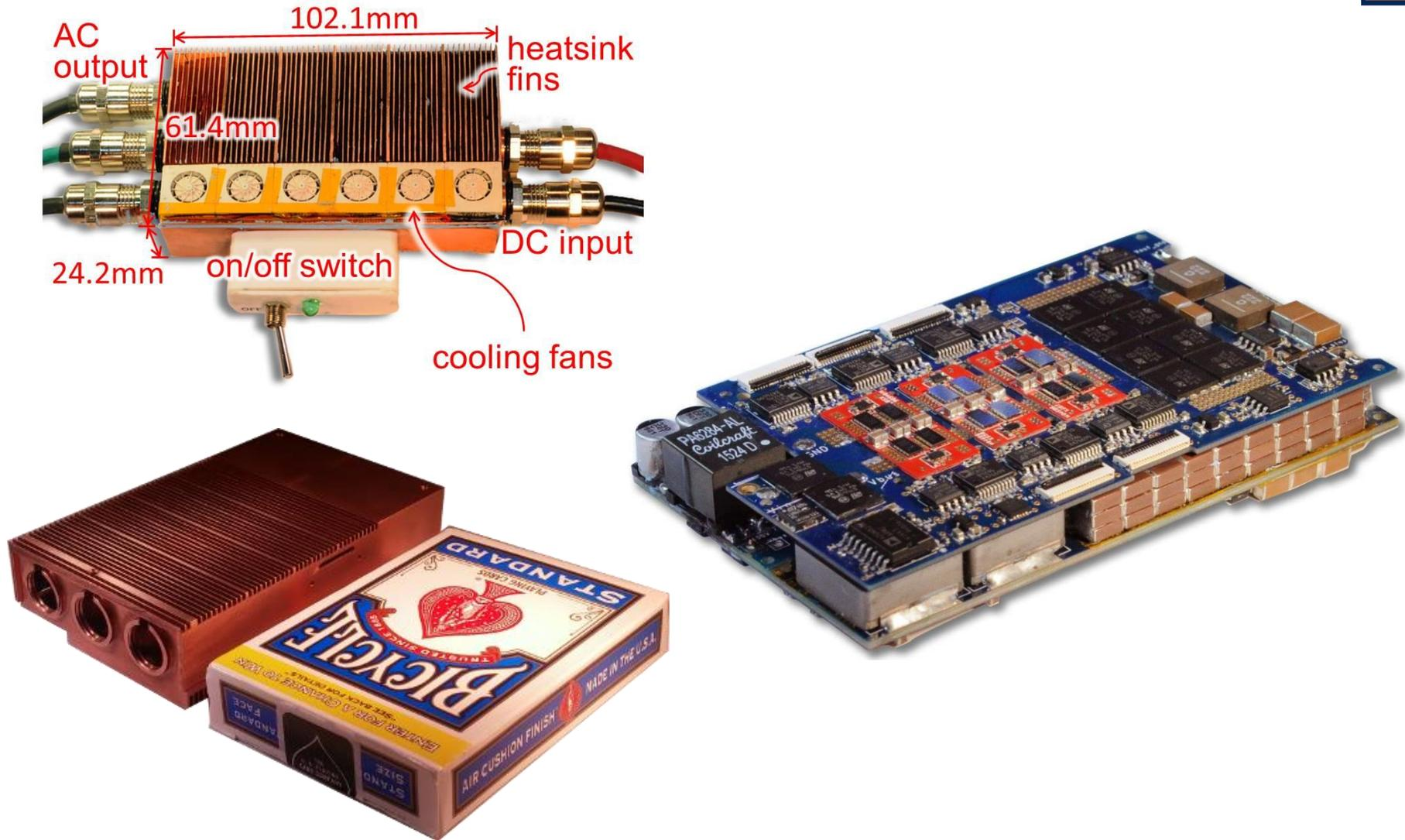
Y. Lei, C. Barth, S. Qin, W.-C. Liu, I. Moon, A. Stillwell, D. Chou, T. Foulkes, Z. Ye, Z. Liao and R.C.N. Pilawa-Podgurski "A 2 kW, Single-Phase, 7-Level, GaN Inverter with an Active Energy Buffer Achieving 216 W/in<sup>3</sup> Power Density and 97.6% Peak Efficiency", IEEE Applied Power Electronics Conference, Long Beach, CA, 2016
