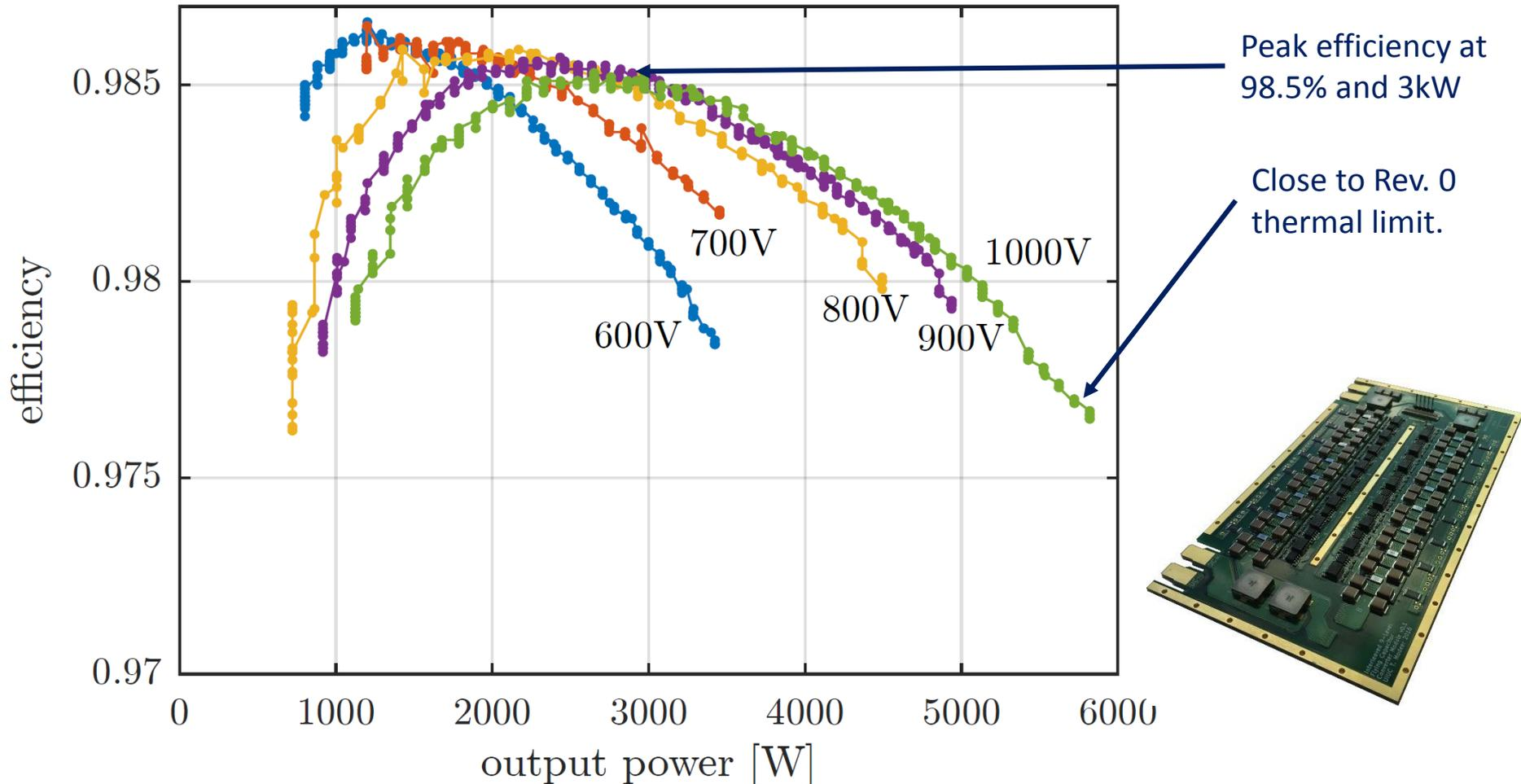
Target: efficiency  $\geq 99.0\%$  at 4.2kW (12 modules @16.7kW)
