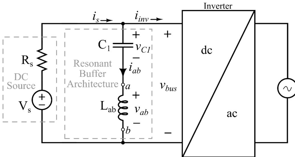
Example: If  $C = 100 \mu\text{F}$  then  $L = 18\text{mH}$  for resonance at 120 Hz
