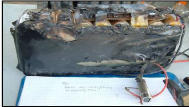
36-cell lithium-ion battery pack with thermal damage.
