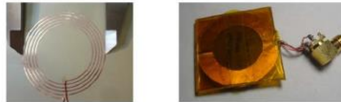
Fig. 3. Fabricated coil and complete receive antenna module for a wearable watch.
