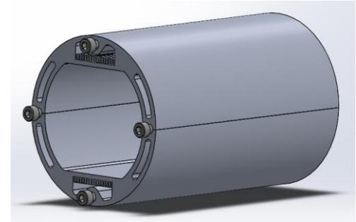
Cylindrical inverter housing for 6-phase inverter.
