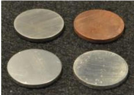
1-inch-diameter copper and Invar coupons: non-plated (top), plated with 4- $\mu\text{m}$ -thick silver (bottom)
