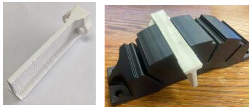
T-shape in-slot heat exchanger.
