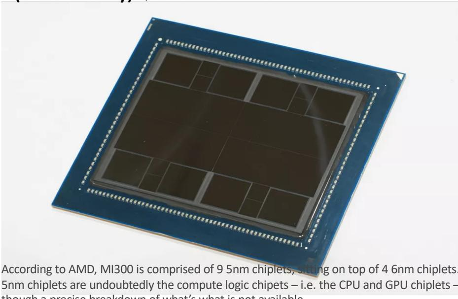
According to AMD, MI300 is comprised of 9 5nm chiplets, sitting on top of 4 6nm chiplets. The 5nm chiplets are undoubtedly the compute logic chiplets – i.e. the CPU and GPU chiplets – though a precise breakdown of what's what is not available.
