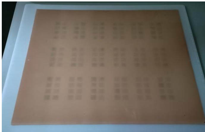
PP with vias (no conductive paste)
