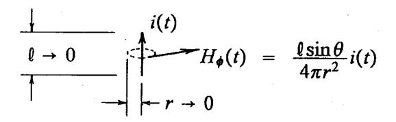
And, with a propagation rate equal to c, the speed of light, it would seem that, if r >> 0
