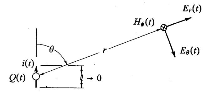
$$E_r(t) = \frac{Z_0c}{4\pi r^2} \left[ Q(t-r/c) + \frac{r}{c} \frac{\partial Q(t-r/c)}{\partial t} \right]$$
