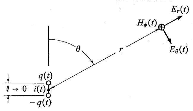
$$E_r(t) = Z_0 \frac{2\ell \cos \theta}{4\pi r^2} \left[ \frac{c}{r} q(t - r/c) + \frac{\partial}{\partial t} q(t - r/c) \right]$$
