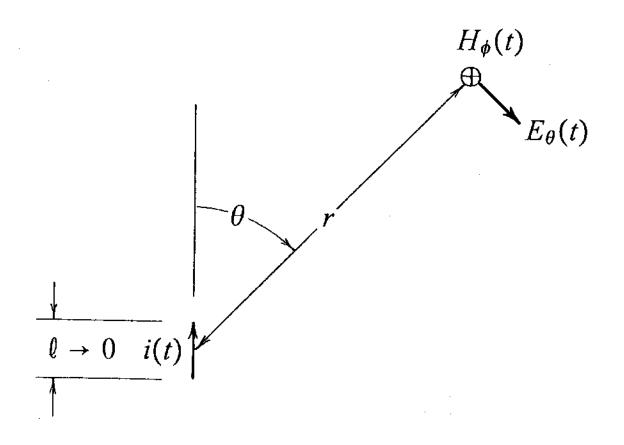
$$H_{\phi}(t) = \frac{\ell \sin \theta}{4\pi r^2} \left[ i(t - r/c) + \frac{r}{c} \frac{\partial i(t - r/c)}{\partial t} \right]$$
