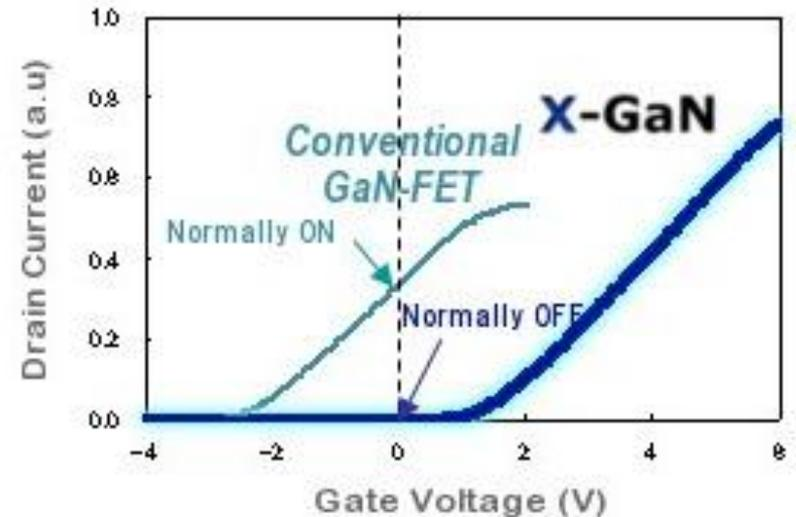
Panasonic makes normally-off by using P type GaN on the gate and discharge in the channel under the gate.
