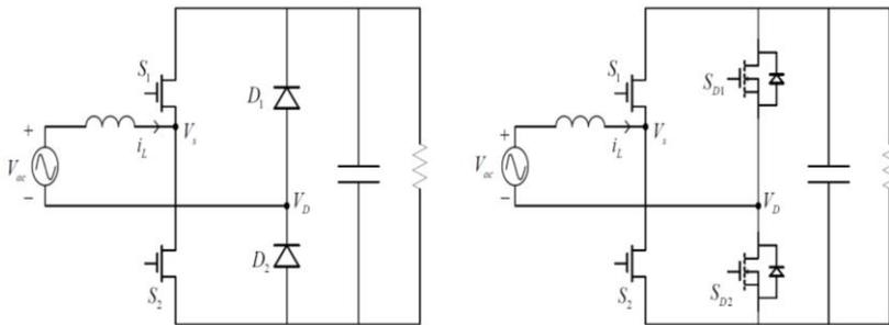
Fig.1 Totem-pole bridgeless PFC boost converter based on GaN HEMT (a) Diode for line rectification (b) MOSFET for line rectification
