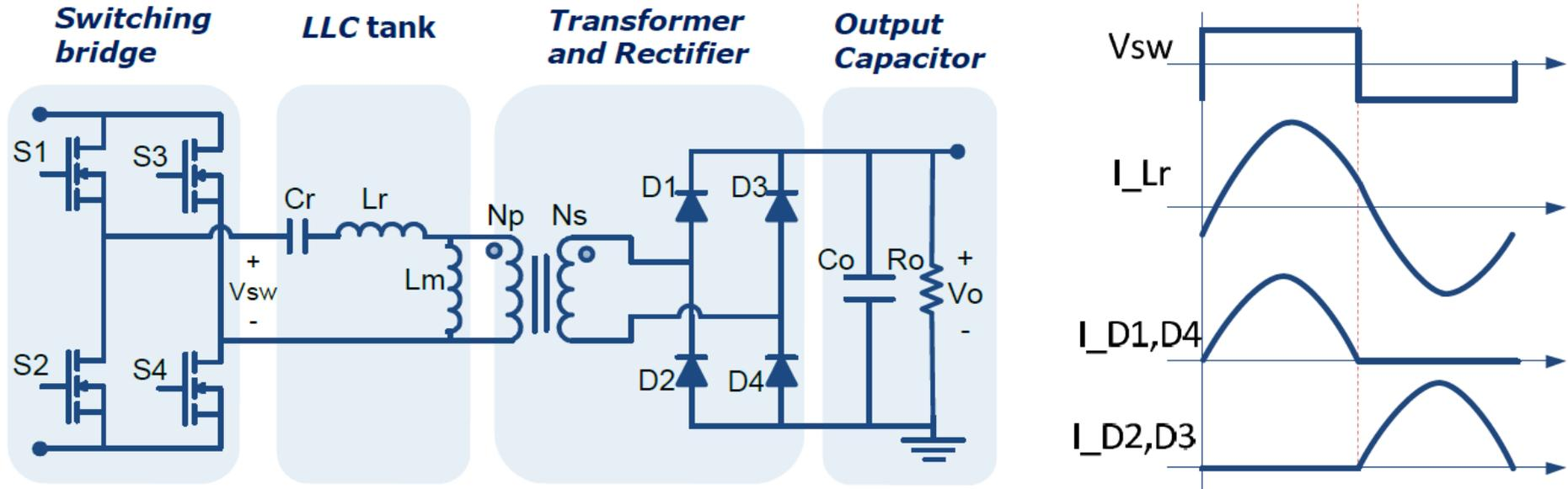
Figure 2.1 Full-Bridge LLC converter with Full-Bridge rectifier
