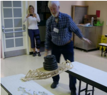
A MASSIVE TRUSS THAT CARRIED 75 LBS WITH HARDLY ANY SAG!
